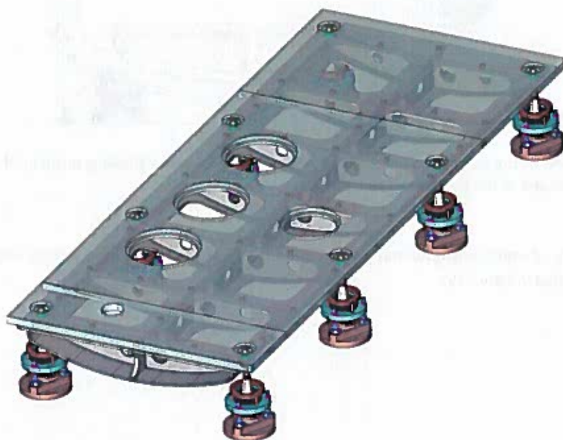
Figure 7: Concept of the internal optical table. The table is composed of three sections sitting on a high-stiffness frame supported by 8 support posts equipped with a bellows system to provide full isolation from the vacuum chamber body.
