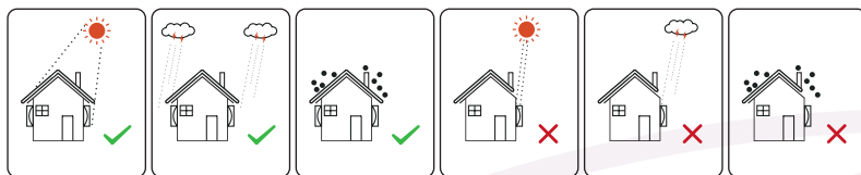
Figure 4-1 Recommended installation location
