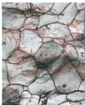
EBSD maps showing grain rotation and matching grain orientation from aluminum alloy sample after loading
