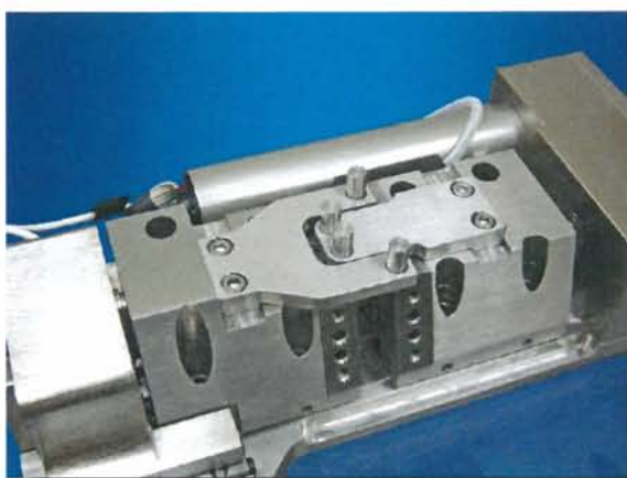
MTEST 2000ES fitted with optional BH 2000E horizontal 4-point bending clamps
