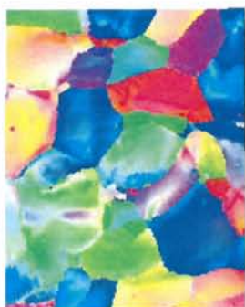
EBSD maps showing grain rotation and matching grain orientation from aluminum alloy sample after loading
