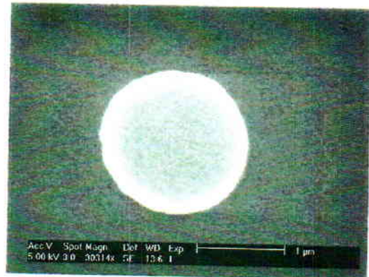
1.5µm diameter permalloy micro-structure (after metallisation and lift-off)
